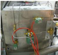
Figure 3: Three computer controlled solenoid valves are mounted to the back of the helium purity meter to automate readings.
