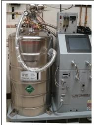
Figure 2: A helium purity meter is attached to the chassis of the Cryomech Liquid Helium Plant 22.
