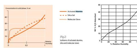
Activated alumina was chosen over silica gel, activated charcoal, and zeolites/molecular sieves. At low relative humidity, the case for recovered helium, zeolites are the most efficacious for adsorbing water. However, the extremely high bake temperature (>300C) makes regeneration difficult. Activated alumina is better than silica gel at low relative humidity and regenerate at relatively low temperatures, >150C. Also, the water capacity of activated alumina is high.
