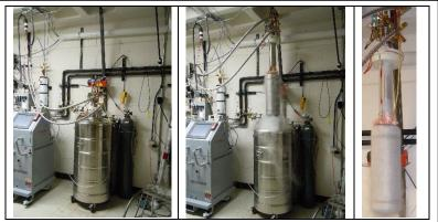
Figure 6: The cold trap is removed from the liquid nitrogen bath.
