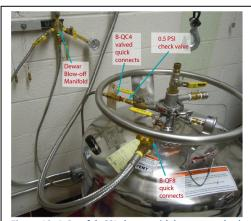
Figure 19: A Cryofab 60L dewar with hoses attached to the vent and exhaust ports. The 0.5 PSIG relief valve has been replaced with a 2 PSIG check valve.
