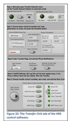
A liquid helium transfer from the LHeP22 150L dewar to a 100L or 60L mobile dewar is automatically shut-off if either the mobile dewar is full, the temperature at the mass flow meter is too low, or the LHeP22 is nearly out of liquid helium. The operator is then notified.
