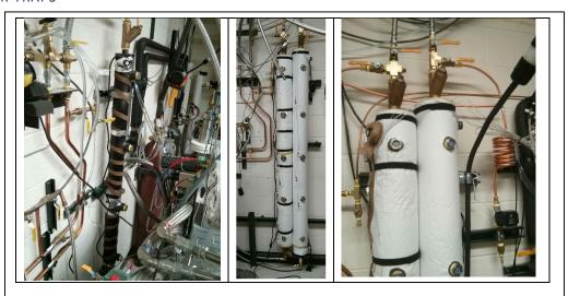
Figure 5: The water traps are filled with activated alumina. (left) A water trap with the fiberglass insulation removed reveals the silicone heater tapes and thermostats. (center) The two traps are mounted side-by-side. (right) Helium gas enters the top of the traps and exits the bottom. During regeneration, a counter flow of air enters the bottom of the trap and exits the top of the trap. This exhaust gas is routed through a cooling coil and then a motorized ball valve.
