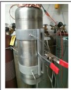
Figure 7: Two band clamp heaters quickly warm the cold trap and prevent excessive icing during regeneration.
