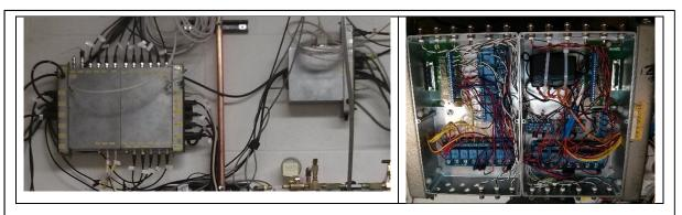
Figure 30: (Left) Electronics box #2 is the larger box on the left, and electronics box #1 is the smaller box on the right. (Right) Inside electronics box #2 are two DB-25 screw-terminal connector blocks, three 8-channel relay boards, three 4-channel k-type thermocouple amplifiers with virtual cold junction offset correction, three dc power supplies, and two 6-outlet power strips.
