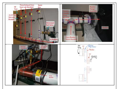
Figure 21: Pictures show (a) the Bladder room manifold, (b) the Bladder room manifold interface with the bladder, and (c) the Bladder send line to the Liquefier manifold showing the pressure transducer and connectors. (d) A sketch of the custom-designed bladder flange assembly.
