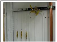
Figure 27: Lab dewar blow-off manifold
