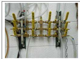
Figure 25: Pressurization/vent manifold
