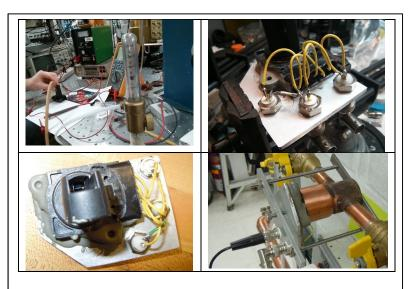
Figure 16: Modified automotive Mass-air-flow sensors are used as adjustable helium flow sensors and the Laboratory and Liquefier manifolds
