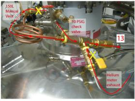
Figure 13: (a) The purified gas enters the liquefier input assembly on the 150L dewar. The point marked "12" corresponds to the same point on the liquefier manifold diagram in Figure 10. (b) The 150L dewar liquefier exhaust assembly sends gas to point number "13" on the liquefier manifold diagram in Figure 10. The coil allows for thermal expansion and contractions without stressing rigidly attached joints.
