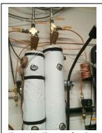
Figure 11: The top of each water trap has an input isolation valve (top) and a manual exhaust port valve (side).
